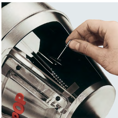
Manually place 6 - 8 blind rivets into the runner on the feeder
